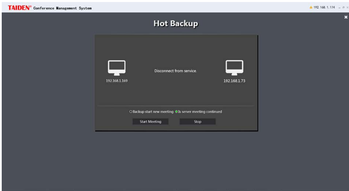
Figure: Software Hot-spare Dual Server
