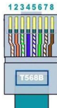
Wiring order (1-8) according to T568B standard: white-orange, orange, white-green, blue, white-blue, green, white-brown, brown
