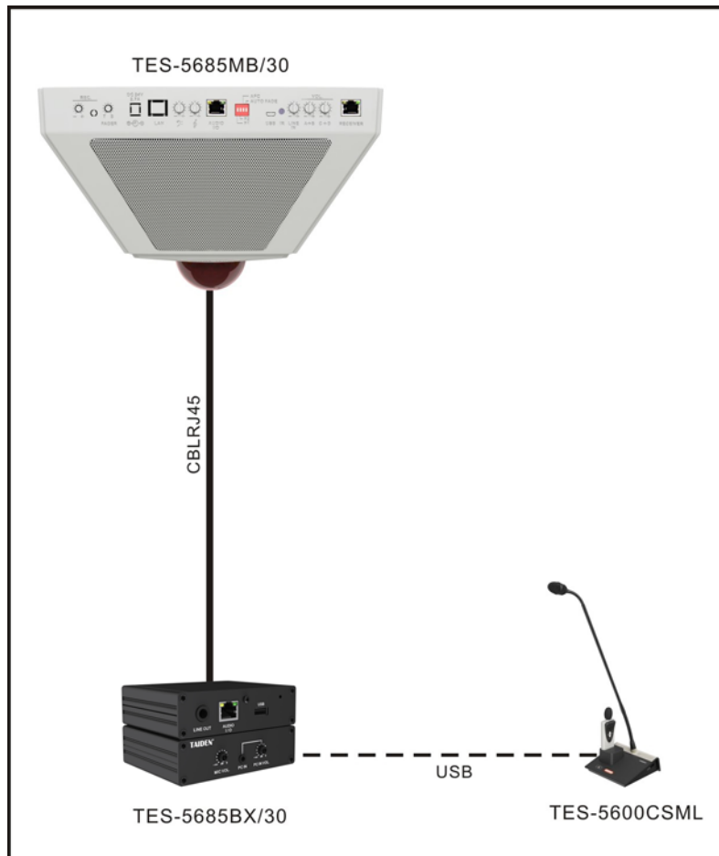
Figure 2.10 TES-5685MB digital infrared classroom audio system
