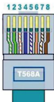
Wiring order (1-8) according to T568A standard: white-green, green, white-orange, blue, white-blue, orange, white-brown, brown
